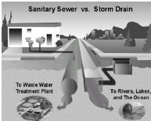
The **Sanitary Sewer System** collects wastewater from indoor plumbing such as sinks, toilets, washing machines, and floor drains where it is transported through underground pipes to a sewage treatment plant. The treatment plant removes many pollutants from wastewater before it is discharged back into a river.
