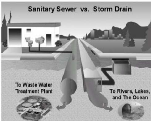
The **Sanitary Sewer System** collects wastewater from indoor plumbing such as sinks, toilets, washing machines, and floor drains where it is transported through underground pipes to a sewage treatment plant. The treatment plant removes many pollutants from wastewater before it is discharged back into the river.
