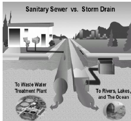
The **Sanitary Sewer System** collects wastewater from indoor plumbing such as sinks, toilets, washing machines, and floor drains where it is transported through underground pipes to a sewage treatment plant. The treatment plant removes many pollutants from wastewater before it is discharged back into a river.
