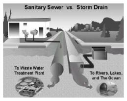
The Sanitary Sewer System collects wastewater from indoor plumbing such as sinks, toilets, washing machines, and floor drains where it is transported through underground pipes to a sewage treatment plant. The treatment plant removes many pollutants from wastewater before it is discharged back into a river.
